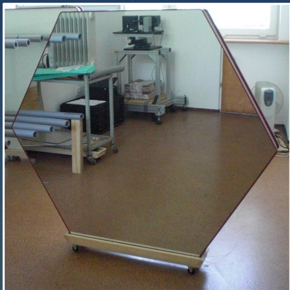
Glass-aluminum composite mirror for MST. Size: 1.2 m (ftf), Focal length 16.14 m, PSF < 20 mm
