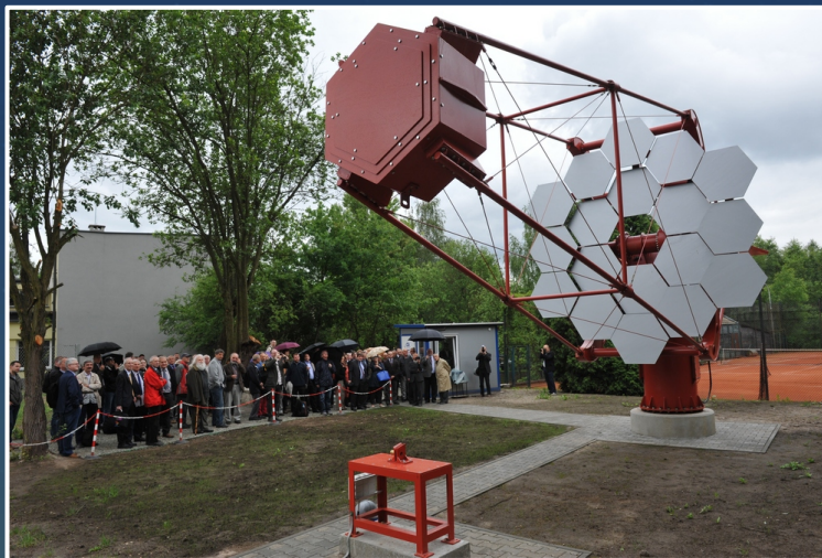
SST-1M; inauguration in June 2014 at the test site in IFJ PAN, Kraków. Dish size: 4 m, Focal length 5.6 m, 18 spherical mirrors Field of view 9.1° Silicon photomultipliers based camera with fully digital readout electronics [DigiCam]; 1296 pixels
