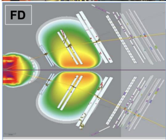
The forward detectors around a toroidal field
