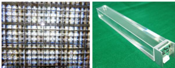
Figure: PHOS cell matrix[left];  $PbWO_4$  crystal, APD(Avalanche Photo Diode) detector and preamplifier[right]
