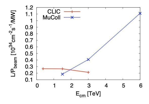
Luminosity normalised to the beam power and as a function of the centre-of-mass energy comparison of the Compact Linear Collider (CLIC) and a muon collider
