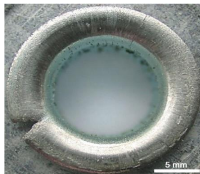
Macroscopic observation of the cracking area of the rivets
