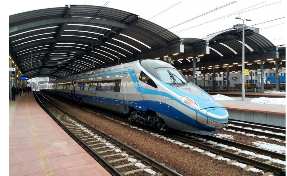
High-Speed ICE Pendolino train, max. speed 250 km/h
