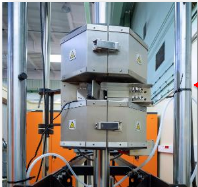
Three-Heating zone split furnace Nominal maximum specimen temperature: 1000°C
