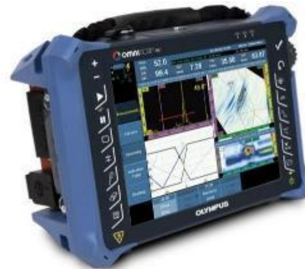
UT Defectoscope Olympus OMNISCAN MX2
