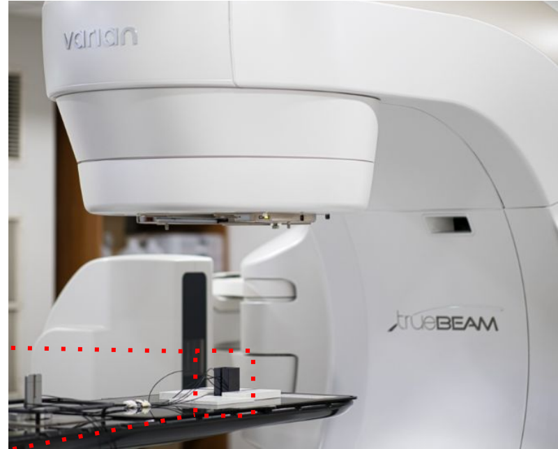
Detector prototype as a tower of cells within the printed enclosure
