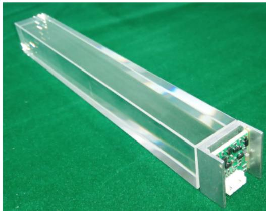
Figure: A detector element consisting PbWO<sub>4</sub> crystal, APD(Avalanche Photo Diode) detector and preamplifier
