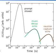
Neutrons capture on hydrogen and product 2.2MeV gamma. In seawater, 33% of neutrons capture on CI; the emitted gamma rays have 8.6 MeV, making the neutron echoes more visible
